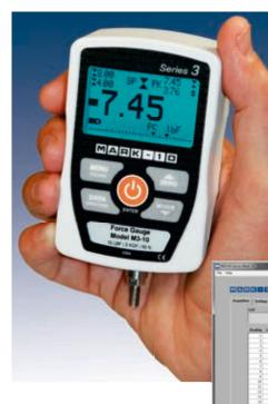
Series 3 digital force gauges are designed for tension and compression force testing in numerous applications from 0.12 lbF to 500 lbF (0.5 N to 2500 N). The gauges feature a sampling rate of 2,000 Hz, producing accurate results under a wide range of test conditions. A backlit graphic LCD displays large characters, and a menu is available to access the gauges' features and configurable parameters. USB output is provided for data collection purposes.
