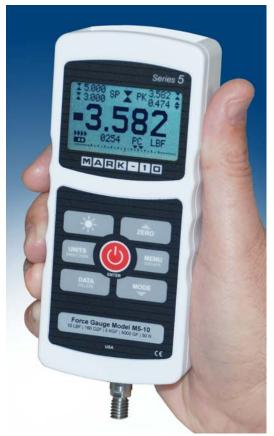
Series 5 advanced digital force gauges are designed for tension and compression force testing in numerous applications across virtually every industry, with capacities from 0.12 lb to 500 lb (0.5 N to 2500 N). The gauges feature an industry-leading peak sampling rate of 7,000 Hz, producing accurate results even for quick-action tests. Accuracy is  $\pm 0.1\%$  of full scale  $\pm 1$
