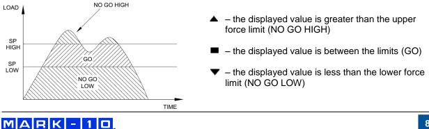
Note: Set point indicators reference the displayed reading, not necessarily the current live load.
