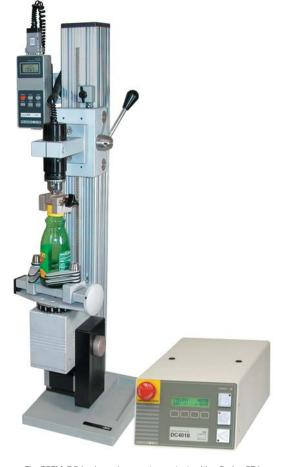
The TSTM-DC is shown in a cap torque test, with a Series STJ torque sensor, BGI force/torque indicator, and G1023 universal closure grip, and G1053 cap grip
